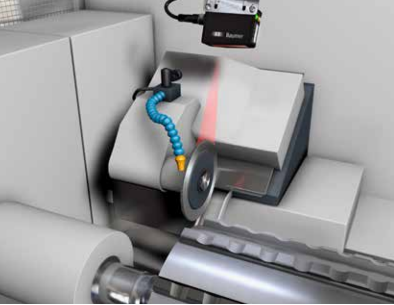
Measurement of the diameter of a grinding wheel in a CNC machine
