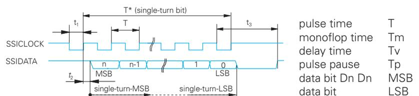
In the idle state the data and pulse lines are at High level. The transfer begins with the first trailing edge. With each following rising edge, the data bits are output consecutively to the data line. The transfer begins with the MSB. If the number of pulses is higher than the number of data bits, only zeros are sent after the data bits.
